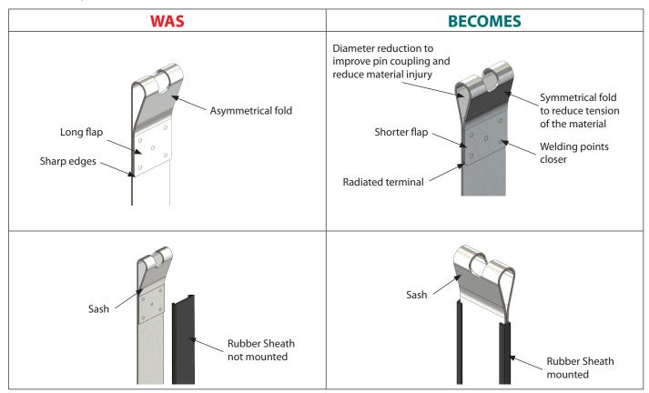
The assembly kit codes remain unchanged as indicated in the catalogue. However, these changes have made it necessary to create new spare parts codes as indicated in the table below:
